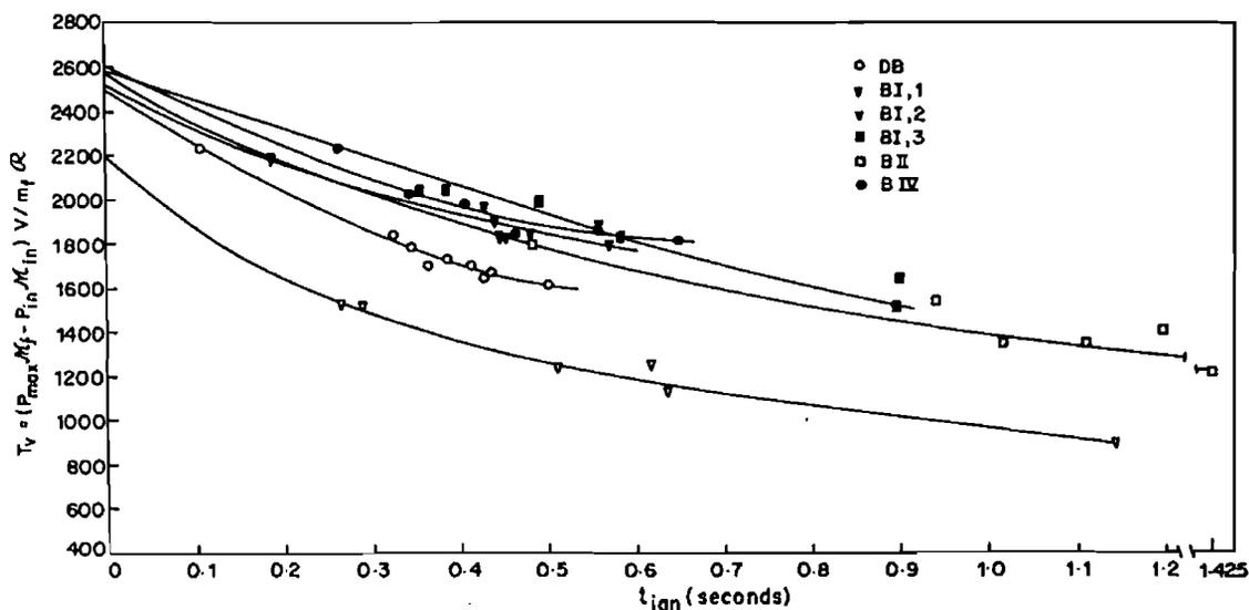
FIG. 6. Plot of  $T_v$  vs  $t_{ign}$  for double base (DB) and composite propellants.
