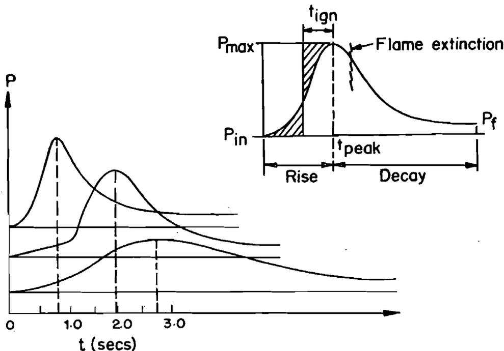
FIG. 3. A typical set of pressure time traces with nomenclature.
