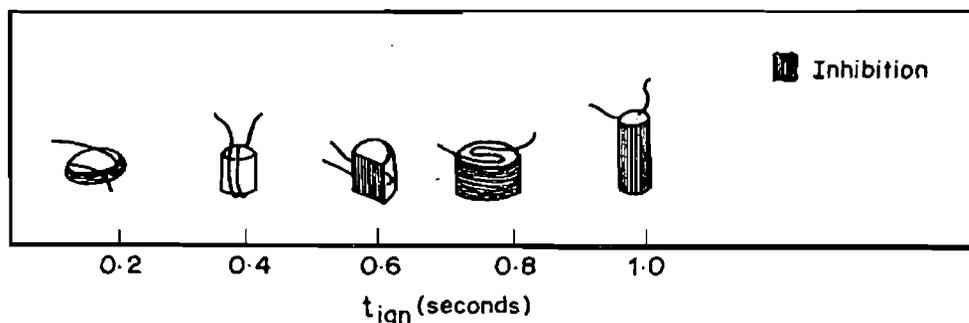
FIG. 2. Methods of arranging the sample to obtain a variety of initial pressure rises (or  $t_{ign}$ ).
